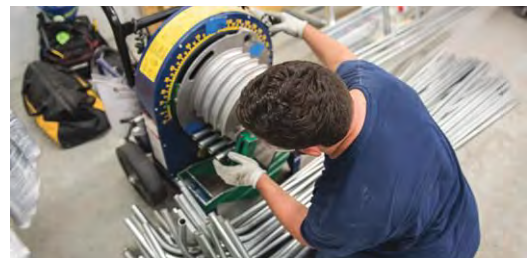
Equipment and materials are prefabricated at Griffin Electric to reduce time and increase quality control.
